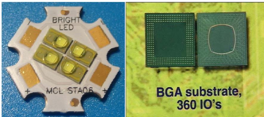
Drilling and metallization of perforations is not required with ALOX™ because the interconnections are made entirely of aluminum and the dielectric material is made of high-quality ceramic. The process is simple, low cost, and requires a limited number of process operations.
